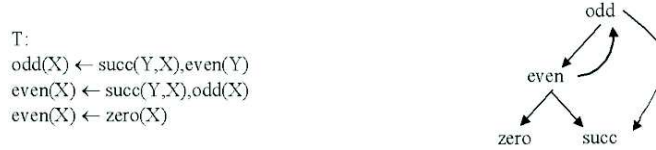
Figure 1. A recursive theory and its corresponding dependency graph for the predicates odd and even .
