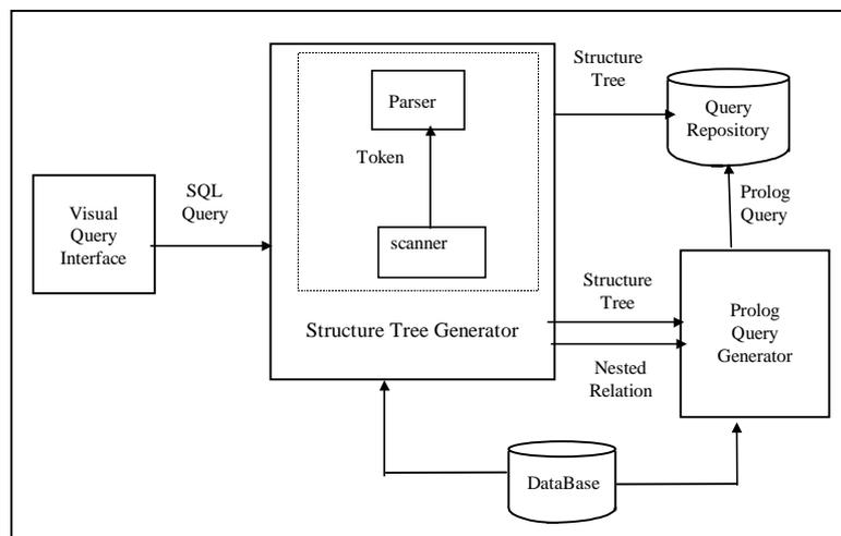
Figure 3. Architecture of the Query Management Tool.
